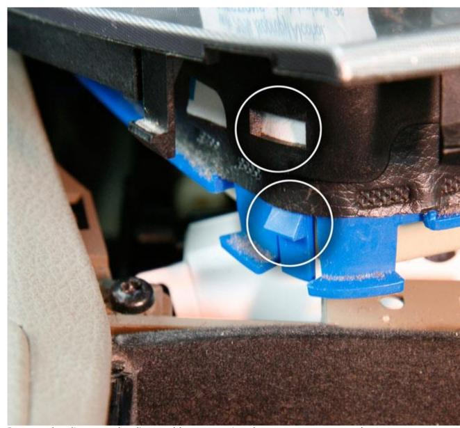
5. Remove the climate and radio panel by unscrewing the two torx screws at the bottom and pulling the bottom of the panel backwards and then downwards.
