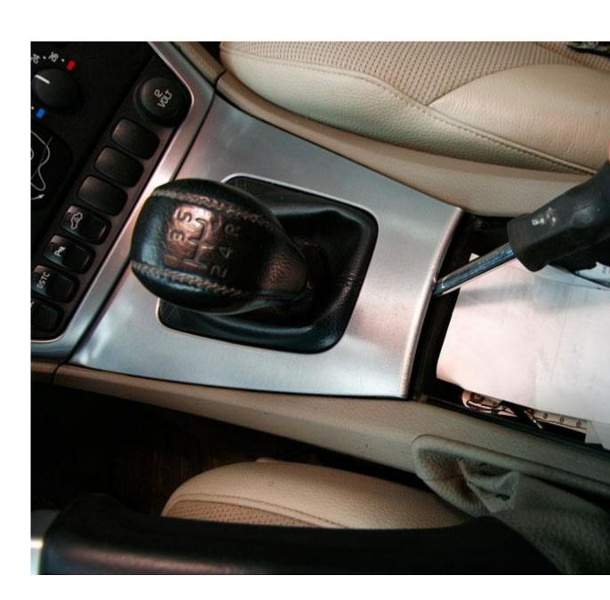
4. Remove the frame by pressing the four blue catches.
