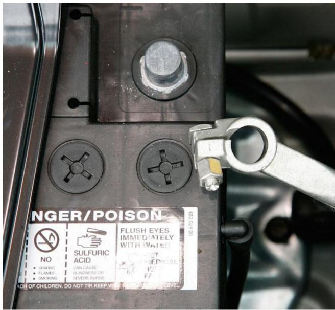
2. Remove the plus/positive connector from the battery, and make sure it cannot come into contact with either the battery or any other part of the car.
