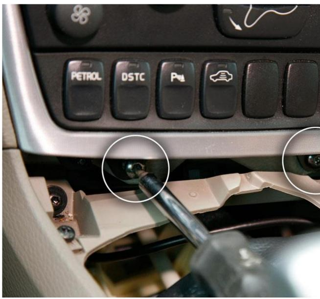
6. Remove the frame by unscrewing the top three torx screws and then unlatching the three catches on either side.
